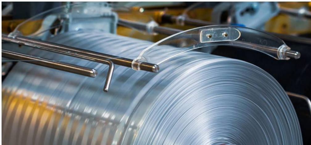
The Cygnet Texkimp creels for polymeric tapes (poly tapes) incorporate unique patented designs for unwinding extruded tapes and monofilaments. Unwinding can occur from a variety of package types with various levels of control and sophistication. Each position is equipped with tension compensation and quick stop braking control, to ensure even running tension and quick stopping without over-tensioning or breaking any of the running ends.
