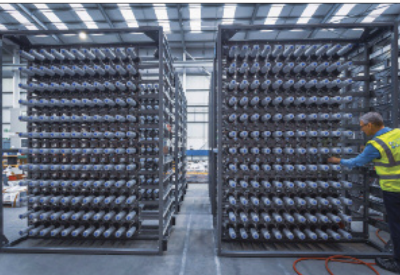
One of Cygnet Textkimp's creels for three-dimensional weaving.
