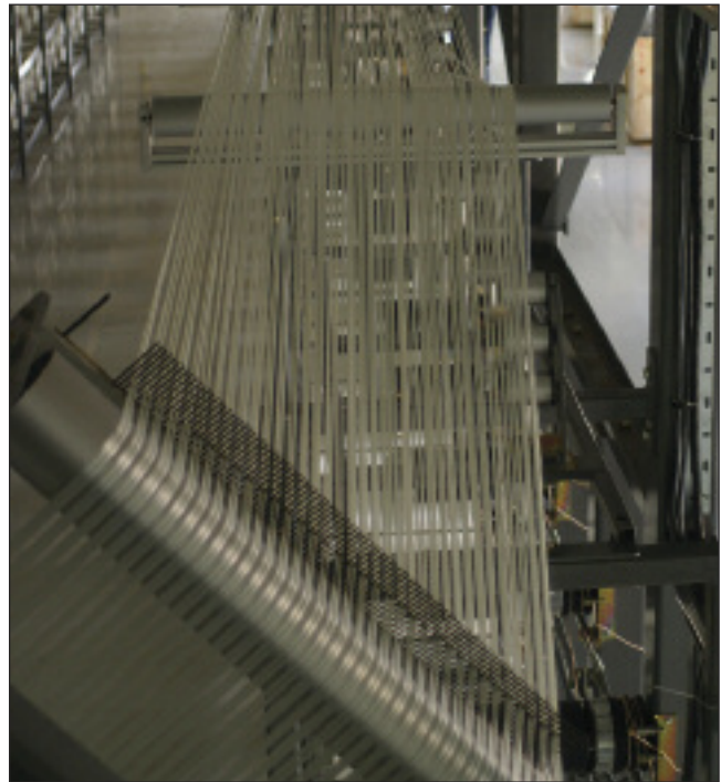
Polyacrylonitrile fibres fed from a creel using an angled guide system.
