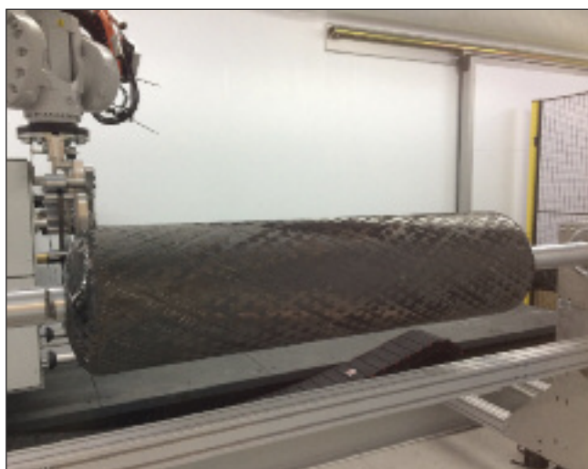
This blank is produced by filament winding and then slit to produce a 1 × 1-m preform.
