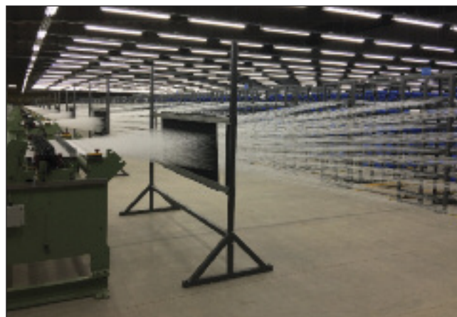
An array of Cygnet Textkimp's creels feeding the looms at a weaving plant.
