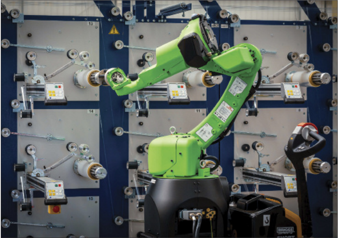
Cygnat Texkimp's collaborative robot is mounted on an automatically guided vehicle (see also, page 36).
