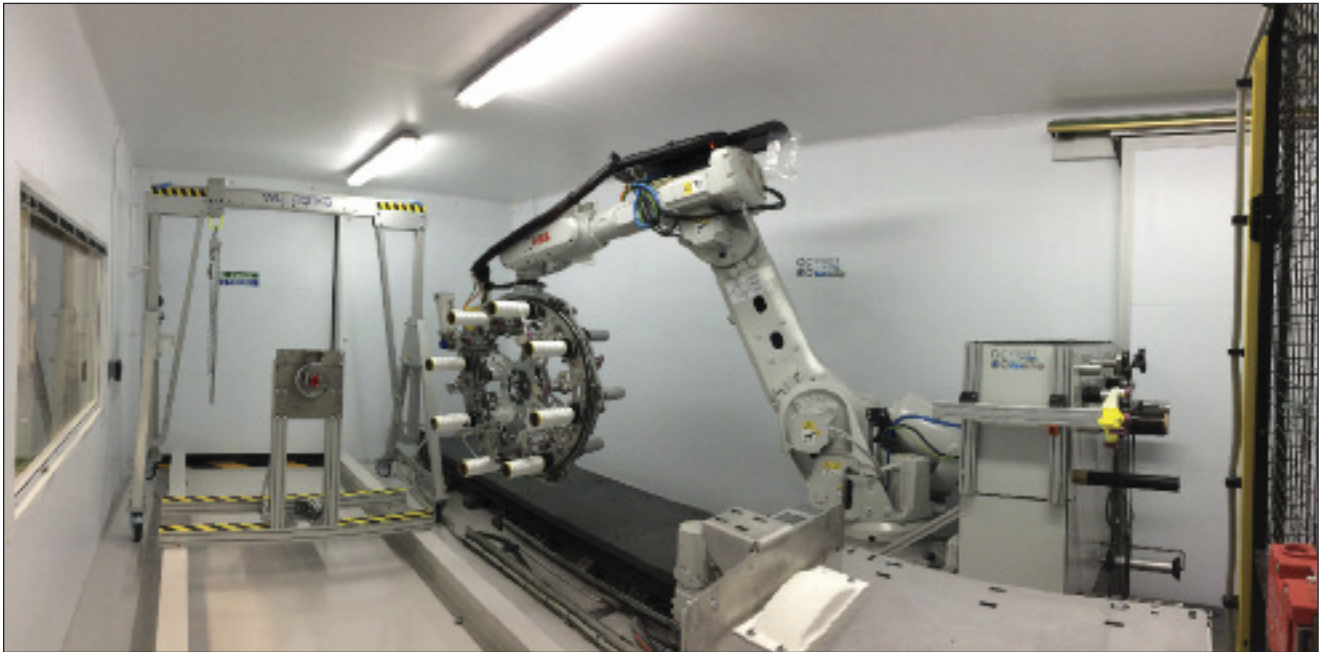
Cygnet Textkimp's 3D Winder is a robotic machine designed to produce complex non-linear parts that vary in cross-section (see also, page 33).
