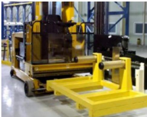
Automated guided vehicles (AGVs) are vehicles that have been programmed to a routine of activities and use sensors to guide their motion through a defined space. The control of the vehicle through routines are updated with information from sensors within the physical space and/or attached to the vehicle. The AGVs can also exchange data and information to and from the factory's physical inventory.
