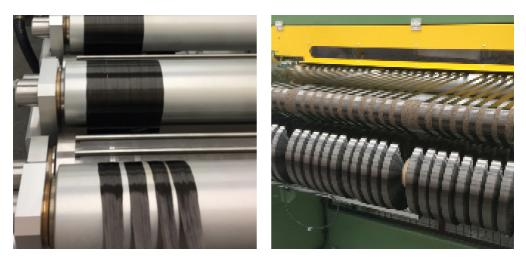
The choice of spreading technique is customised to suit the process and requirements of the fibre in each application. Customization is often achieved through lab testing at our facility.
