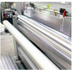
Cygnet Texkimp's Blade and Roll Over roll coating technologies offer a relatively low-cost way of applying high-viscosity coatings with medium to high coat weights, typically 30gsm and above.
