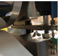
Compactors and Laminators operate by passing a material/substrate (paper, film, fibre, fabric) through a set of rotating rolls.
