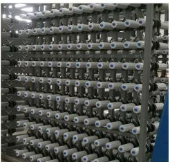
Cygnet Texkimp's state-of-the-art composite creels are designed for the unwinding of high performance multifilament packages into a large range of low and high speed downstream processes.
