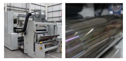
Cygnet Texkimp's embossing technology can be used to process a range of materials, from thin films and foils with a thickness of just 10 microns up to 2mm stainless steel sheets. In-line heating technology can also be incorporated where necessary.
