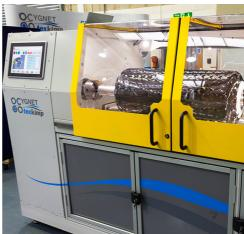
Cygnet Texkimp offer a range of filament winding solutions for processing multifilament tows. Equipment may be tailored to your application, with the number of axes and data input method dependent on component complexity.
