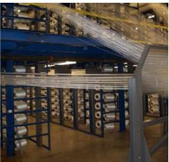
Cygnet Texkimp's Over End creels are designed for unwinding a packages of material from a stationary position.
