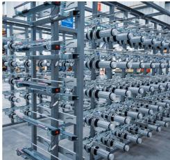
Poly tape creels incorporate unique patented design for the high speed unwinding of yarns, extruded tapes and monofilaments into beamers, dipping lines and other downstream process machinery.
