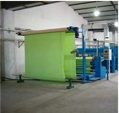
Cygnet Texkimp's Powder Scatter system is most commonly used to apply and fuse a thermoplastic powder to a fabric substrate – typically glass or carbon to create a thermoplastic prepreg or similar product.
