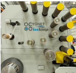
Cygnet Texkimp's Prepreg Tape Slitting technology is designed specifically for use in the composites industry, typically to slit and spool thermoset UD prepregs.
