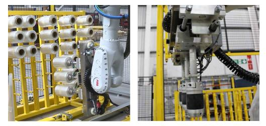
Robotic packaging and handling systems are used to decrease the mount of operator interface required for managing the materials into, or product off, a production line. Automation also enables production systems to work with larger/heavier packages.
