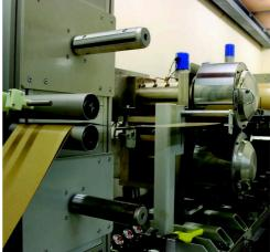
Thermoplastic prepreg lines make use of a polymer system that has reoccurring plasticity with heat.
