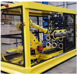
Cygnet Texkimp's Winder Tending Systems are robotic systems used to automatically load fibre unwinds or unload winders.
