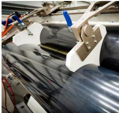
Coating is the physical process of laying a liquid or solid onto the surface of a paper, fibre or fabric. The objective is to achieve uniformity of coverage (uniformity of weight distribution) while controlling the ariance of thickness of the coating.
